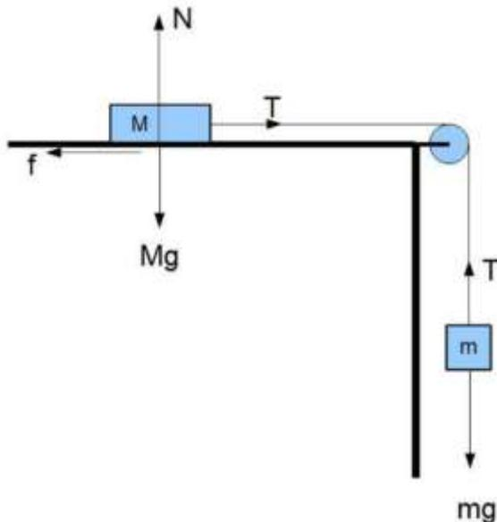
The analysis for the y direction forces acting on the wooden block is the same for both problems.
